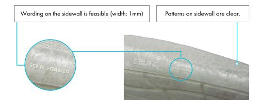
Unique signature bursting effect lines on the flat surfaces, unique to the SCF process.
